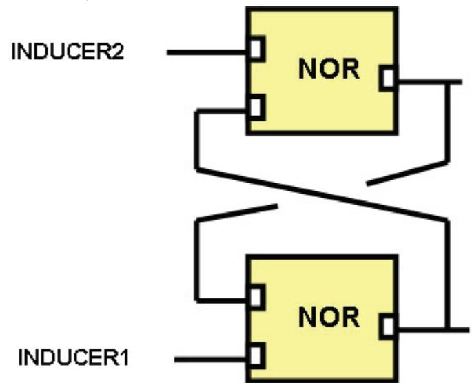
Figure 2. Block diagram for SR latch of Figure 1.
